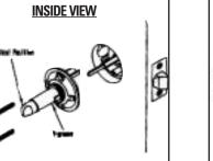
Thread the rose onto the inside adapter clockwise until it is firmly seated against the door surface.
