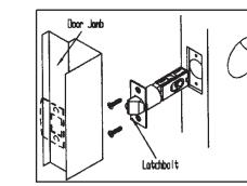
Slide the latch into the door with the angled side of the
